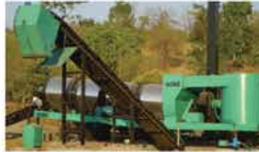
Drum Mix Plant
